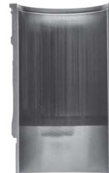
Severely Scuffed Liner
