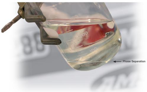
When ethanol/water mixtures fall to the bottom of fuel containers, it leads to lean-burn situations. Quickshot helps keep water molecules dispersed to prevent phase separation.
