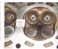
Combustion chamber after P.i. treatment.
